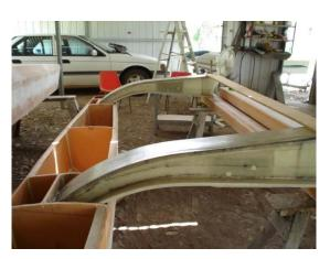
The floats are levelled and the beams are set up through the appropriate bulkheads.
