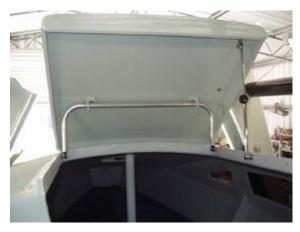
Forward hatch was attached with Sikaflex and stainless screws.
