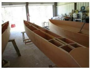
The laminated panels are too stiff to bend over the deck shape. We attached scraps of foam on the outside of the hull to temporarily hold the deck. The foam was joined to the right length and drywall screws were used to attach the deck foam to the hull. Care was taken to not screw into the hull itself. The deck was laminated with glass cloth and resin on the outside. When the glass hardens still attached to the scrap foam. The scraps were removed and the inside of the deck was laminated.
