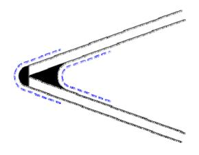
Because it is narrow and difficult to reach, it can be a problem finishing inside the stem. The best way we have discovered is to sand the inside of the bow and use a section of pre-wetted double bias glass laid in as shown below. When the glass hardens resin mixed with aerosil is poured into the gap. This should be done gradually as the resin will generate considerable heat with a possibility of catching fire.
