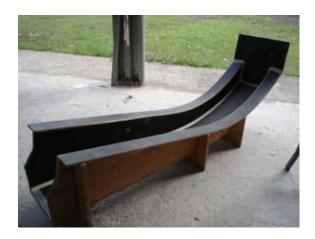
This mould was built using form ply. Form ply is readily available, is relatively inexpensive and has a smooth surface so the glass doesn't stick (but resin coated plywood will work as well).
