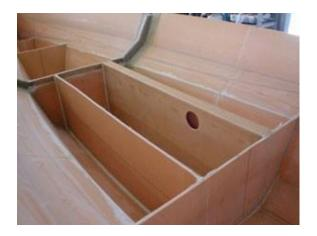
If you want to paint the inside of the lockers it is easier to do that before the floor is installed.
