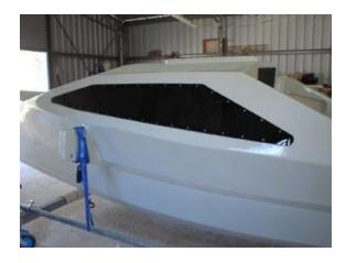
The locker covers are painted, trimmed and attached with hinges. Small pieces of stainless steel are bent and added as latches with some spectra rope added.
