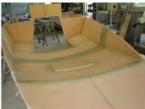
Plywood inserts are added to hold the locker lids.
