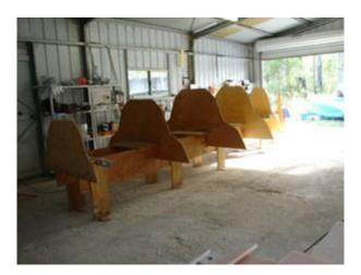
If the boat is to be built using plywood then the sheets are scarfed together and joined to the building frame. The edges bogged and sanded and the glass in laminated over the hull while it is still on the frame.
