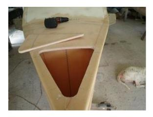
The anchor locker is cut and finished inside. A support to hold the fore stay is added to the forward bulkhead. The foam around the edges is removed, filled and the plywood-insert added hold the anchor lid.
