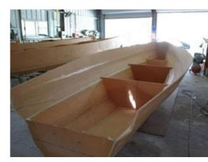
The main beams are taped in. A ring of glass is laminated around the main hull from side to side on the forward and aft beams.
